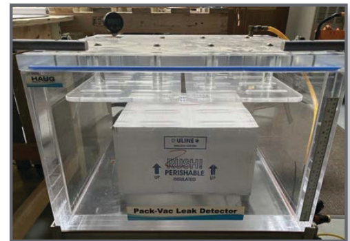
Advanced Labs' vacuum chamber simulates low pressure air travel for packaging flown by plane to assure no bursts or damage occurs.
