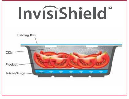
negative organoleptic properties. The InvisiShield<sup>TM</sup> material is extruded and remains stable throughout the supply chain distribution. It contains a base polymer, a channeling agent and the active ingredient (CIO<sub>2</sub>). The release kinetics of the CIO<sub>2</sub> is triggered by relative humidity in the package. CIO<sub>2</sub> then migrates through the same channels or through the polymer blend itself into the surrounding environment in a controlled manner.
